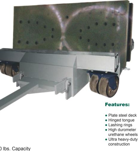
Green Valley can supply trailers for moving heavy loads throughout the manufacturing area. The unit shown features a drop deck design for a low load center of gravity. This unit has a 50,000 lb. capacity, but can be increased or decreased to suit the customer's need. Custom tow bars and several additional options are available.
